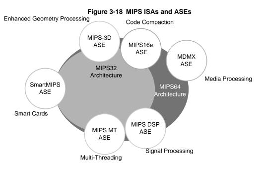
The MIPS32 Architecture is a strict subset of the MIPS64 Architecture. ASEs are applicable to one or both of the base architectures as dictated by market need and the requirements placed on the base architecture by the ASE definition.
